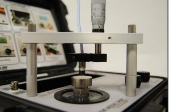
Eddy current proximity probe static and dynamic output checked with the 9100-PPA01 fixture
